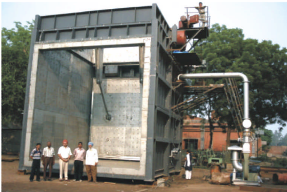
5600mm sq. (GE Frame-9E) Gas Flow Diverter - Toggle Drive, Electric operation
