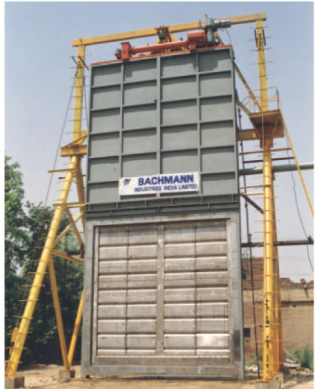
A frame 9E GT guillotine under vertical testing at Faridabad works.
